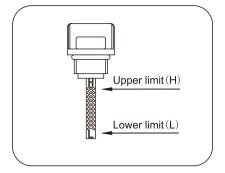
Remove the dipstick again and check oil level. Level should be at top of indicator on dipstick.
