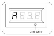
Note: If display value is less than 100,the numeric display will accurate to one decimal place. If the operation time is 100 hour or greater, the display will be "101", "102" and so on.
