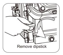
3.Add the oil of the recommended type to the upper limit of the dipstick.
