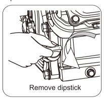
Remove the dipstick again and check oil level. Level should be at top of indicator on dipstick.
