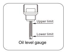
Fill to the upper limit (marked with "H") of the dipstick with the recommended oil if the oil level is low.
