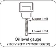
Fill to the upper limit (marked with "H") of the dipstick with the recommended oil if the oil level is low.
