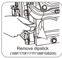
3.Add the oil of the recommended type to the upper limit of the dipstick.
