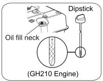
Reinstall and fully tighten the dipstick.
