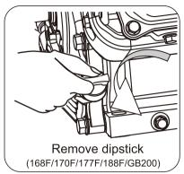
Remove the dipstick again and check oil level, which should be in between the upper and lower limit.
