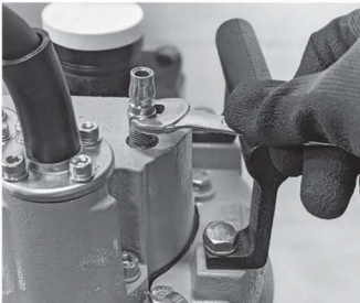
Fig. 1 Quick Coupler Installation.
