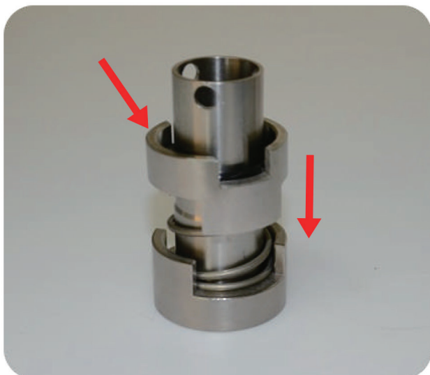
Step4: put the sheath into the shaft
