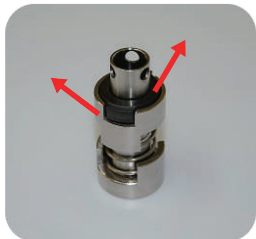
Step6: take rotation of the ring,sheath out
