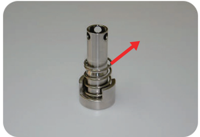
Step8: take compress spring out
