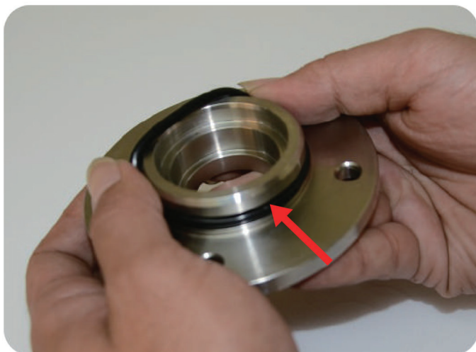
Step6: put O-ring (P44) into the set base of shaft seal
