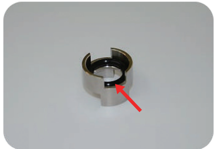
Step3: put the sheath into the O-ring (P26)
