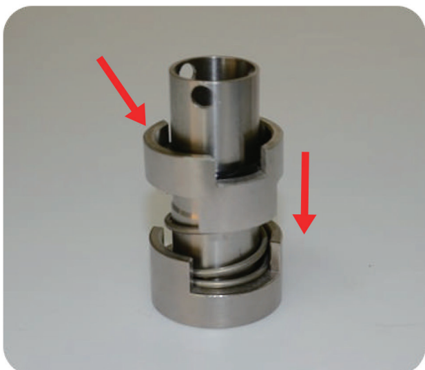
Step4: put the sheath into the shaft
