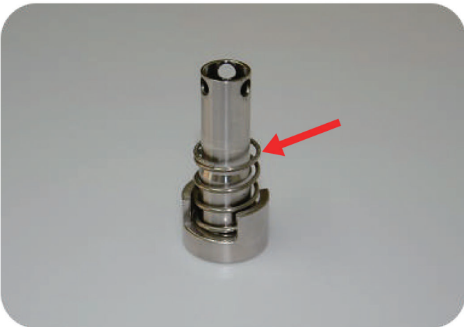
Step2: put the compress spring into the shaft
