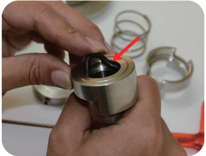
Step1: put O-ring (P22A) into the groove of shaft
