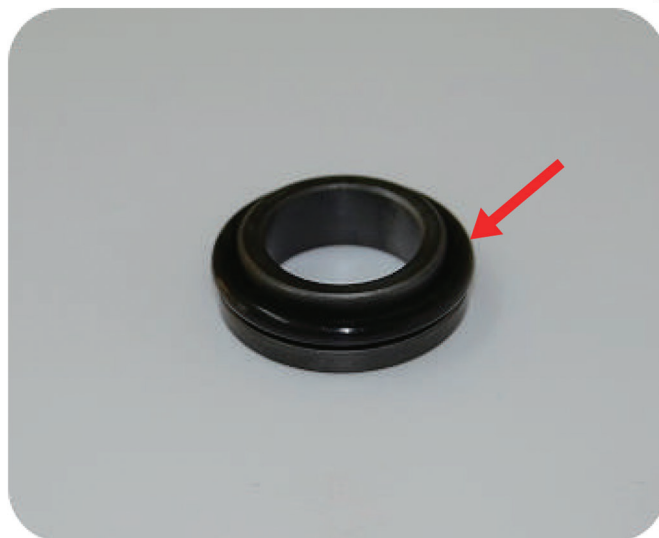
Step7: put O-ring (P32) into the fixed ring
