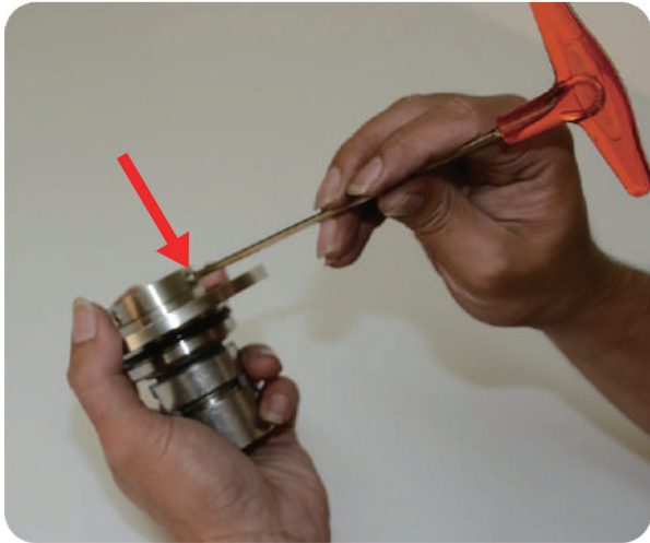
Step1: use 3mm hexagon wrench turn on the bolt
