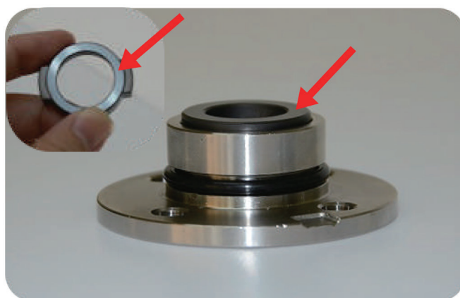
Put the fixed ring smoothly, cannot have difference of height, bright face up
