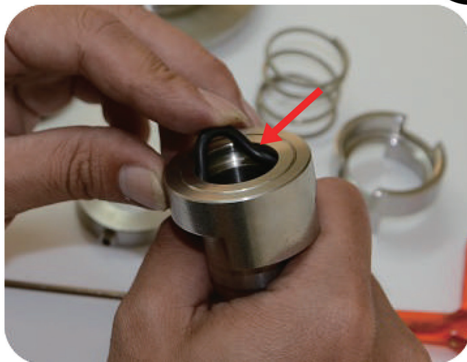
Step1: put O-ring (AS568-114) into the groove of shaft
