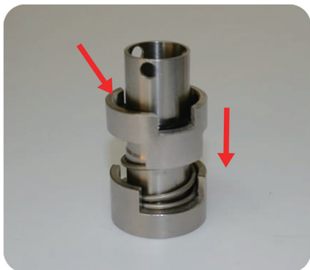
Step4: put the sheath into the shaft
