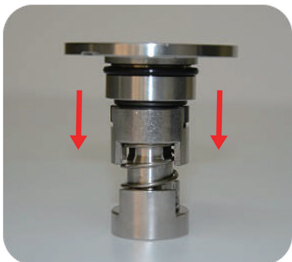
Step9: put the set base of shaft seal on the shaft
