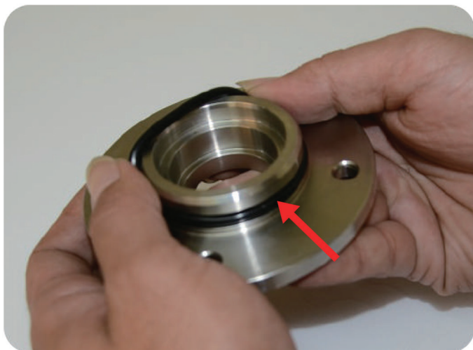
Step6: put O-ring (AS568-123) into the set base of shaft seal
