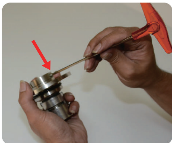
Step1: use 2.5mm hexagon wrench turn on the bolt
