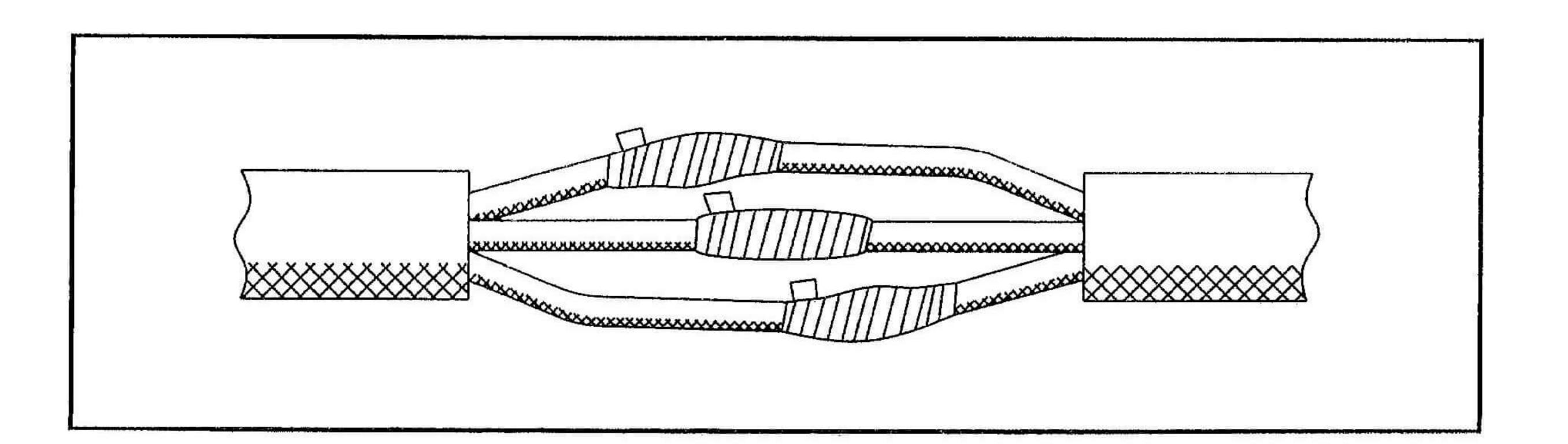
3.8.5 Wrap the cable that is wrapped with the waterproof adhesive tape with the electrical insulating tape.
