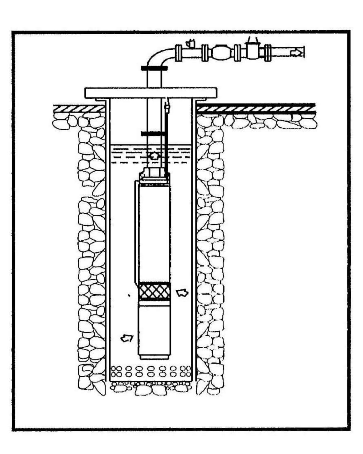
3.6 The electric pump shall be connected to the power source for trial operation before entering into water. The time shall not exceed 3 seconds. The cable lines of single-phase water pump shall be connected according to the wiring diagram on the electric machine or control cabinet strictly with correct colors. The wrong wiring will cause abnormal works or even damage the electric machine; three-phase water pump can be connected without differentiating cable colors.
