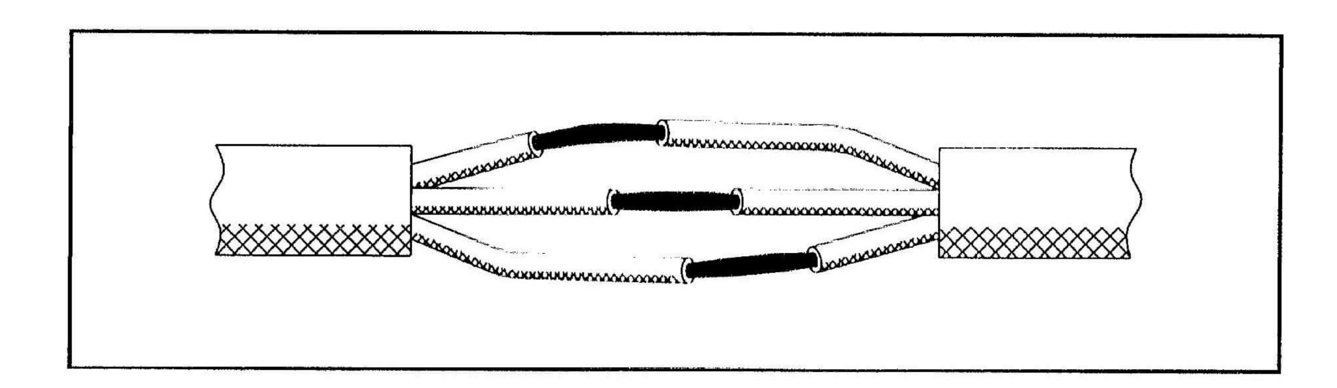
3.8.4 Wrap the cable that is covered withthe electrical insulating tape with a waterproof adhesive tape from the 20-30mm core cord. The waterproof adhesive tape should be 10mmlonger than the electrical insulating tape at both ends. Before the wrapping, the waterproof tape should be stretched out 1-fold its length and follow the normal use.
