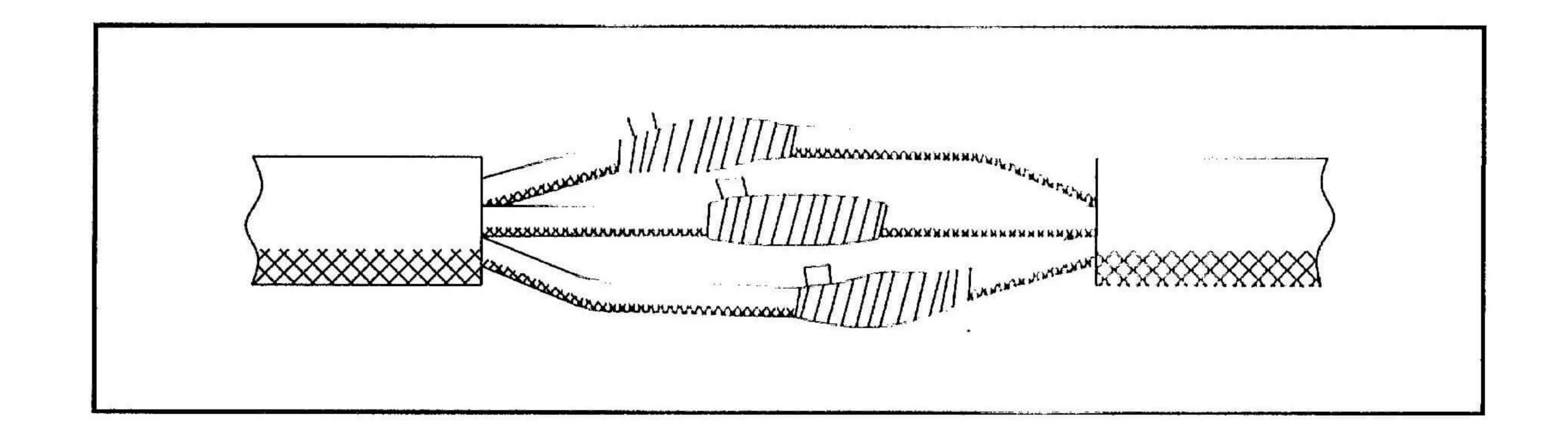
3.8.6 Wrap the cable that is wrapped with the electrical insulating tape with the waterproof adhesive tape. The waterproof adhesive tape should be 10mm longer than the electrical insulating tape at both ends. Before the wrapping, the water proof tape should be stretched out 1-fold its length and follow the normal use.
