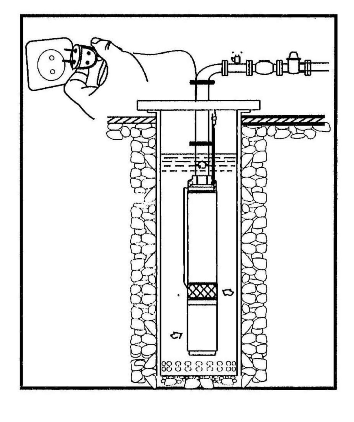
3.7 A power line can be added with rather distant power supply. Please select proper cable lines according to table 1 to avoid too thin cable that will lead to abnormal operation.
