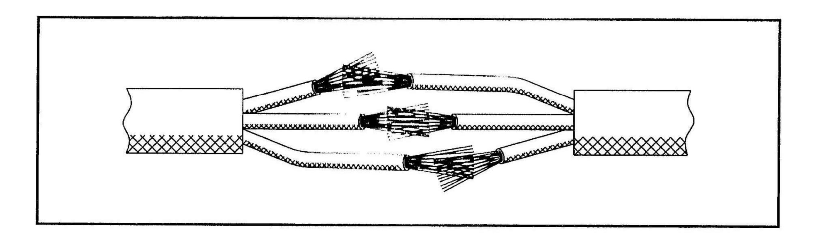
3.8.3 Tightly wind and cover the cable with the electrical insulating tape from the 15-20mm core cord.
