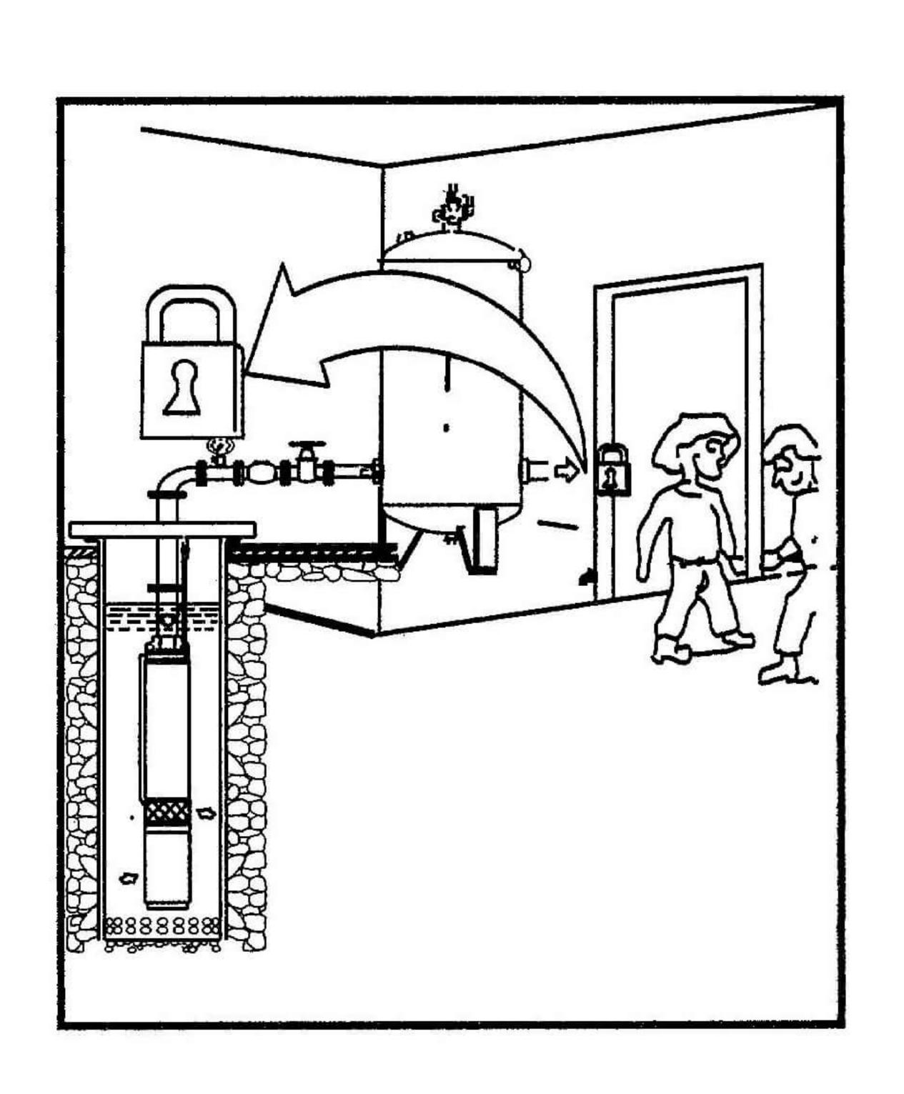
3.4 When the water pump reaches a certen length, the motor and the pump body need to be packed separately. In case of a separate packing, first remove the filter screen and cable protection plate from the pump body, then place the pump body on the motor to make the spindle head of the rotor smoothly slide into the coupling, manually rotate the coupling to check if it can run normally, then screw up the connecting bolt, and finally install the filter screen and cable protection plate.
