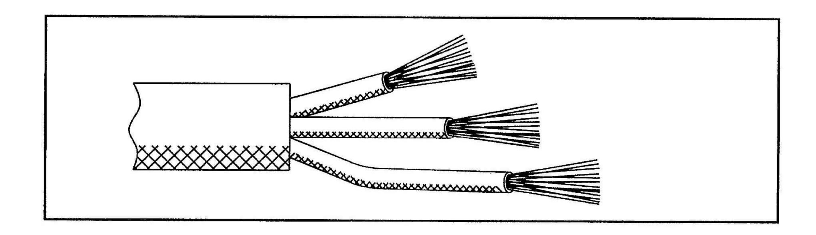
3.8.2 Tighten two cable lines with the same color into spiral shape so as to guarantee close connection;
